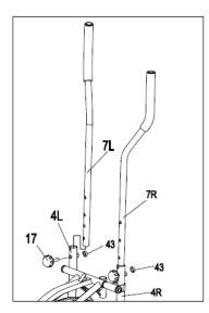
Insert the handle bar (7L/R) to the L/R swing bar (4L/R), select a height setting that is comfortable to the user, and make sure both handle bars are set at the same height. Lock each handle bar in a place with knob bolts (17).
