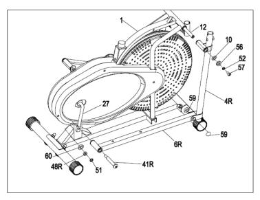
A: Remove allen bolt (57), spring washer (52), D-shaped washer (56), and washer (10) from the long axle (12) on one side, mount one swing bar (4 L/R) to the main section by using the long axle (12), then attach the other side swing bar (4 R/L), and reinstall the washer (10), D-shaped washer (56), spring washer (52) and allen bolt (57) as shown. Please don't fix tightly at this time.
