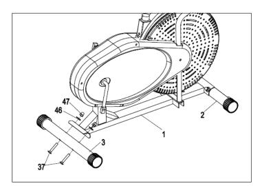
Install the front bottom tube (2) and back bottom tube (3) to the main frame (1) with bolts (37), arc washers (46) and acorn nuts (47).
