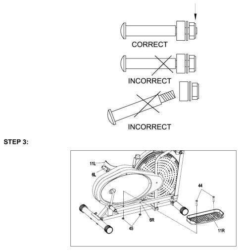
Attach the pedals (11L, 11R) to the pedal tubes (6L, 6R) with bolts (44) and nylon nuts (45).
