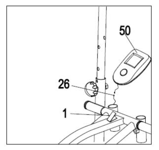
Connect the computer wire with sensor wire (26), after that insert the computer (50) to the main frame (1).
